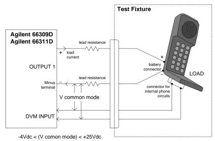
Figure 3-7. DVM Measurement Example
